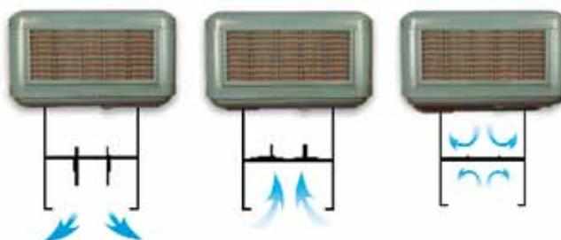
Weather Seal open allows cool air into your home when air conditioner is in use.
